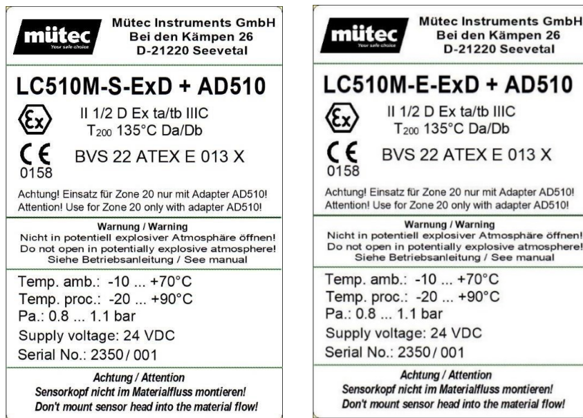
Fig. 7 Type plates of the microwave sensors for zone 20
